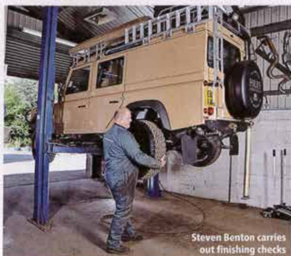
Highly sprung, twin rear shocks and heavy duty springs
